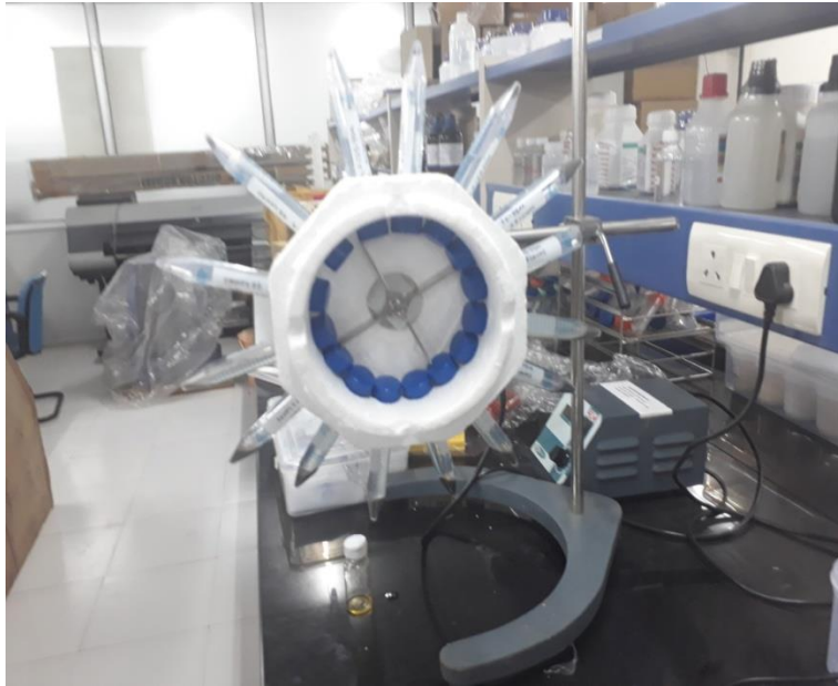
Figure 10. Stirrer used for continuous agitation of samples
