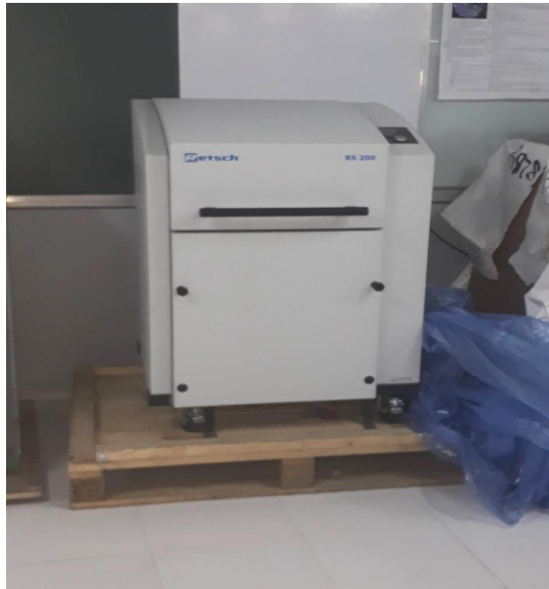
Figure 7. Photograph of the grinding machine (Retsch RS200)
