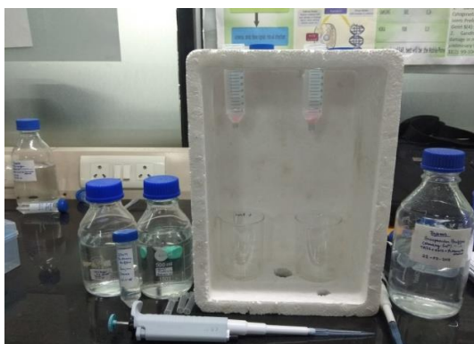
Figure 3.3. The Setup of Affinity Chromatography
