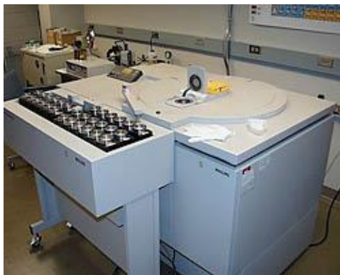
Fig 18:-An XRF spectrometer, with the sample port on top, and a set of samples in silver metallic holders in the sample changer in front. (Source https://serc.carleton.edu/research_education/geochemsheets/techniques/XRF.html )
