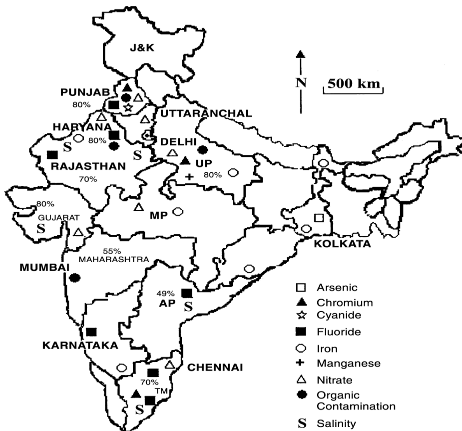
Figure 2.1 Contaminants in ground water of India (Chaudhary et al. , 2002)
