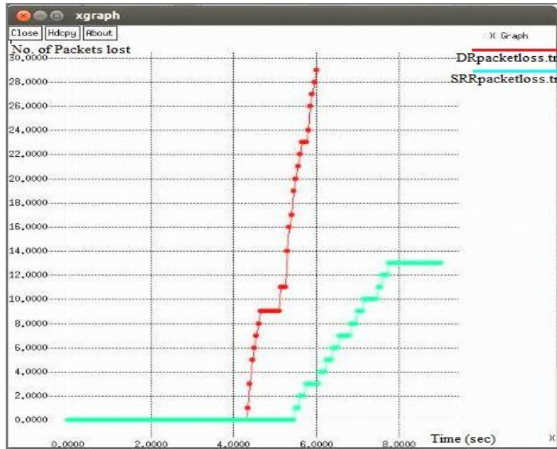
Fig. 6.14 Graph- Comparative graph of Packets lost v/s Time in existing and proposed work
