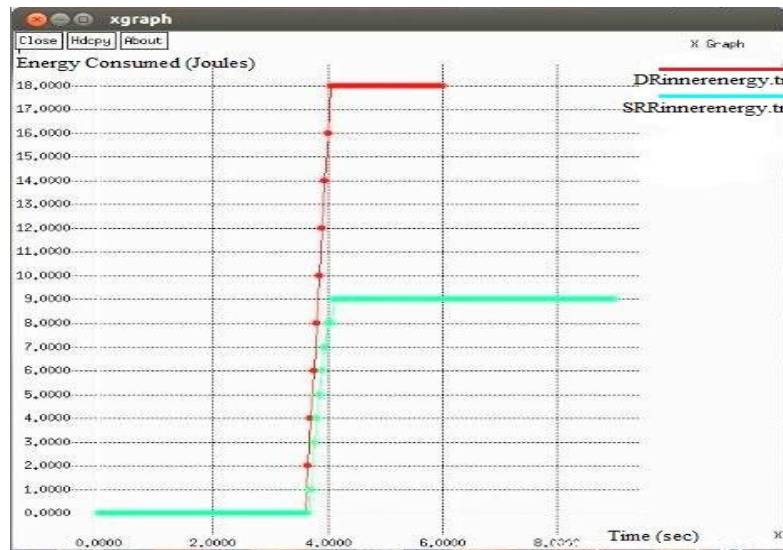
Fig. 6.6 Graph- Comparative graph of inner region showing Energy Consumed v/s Time graph of Existing and Proposed Work
