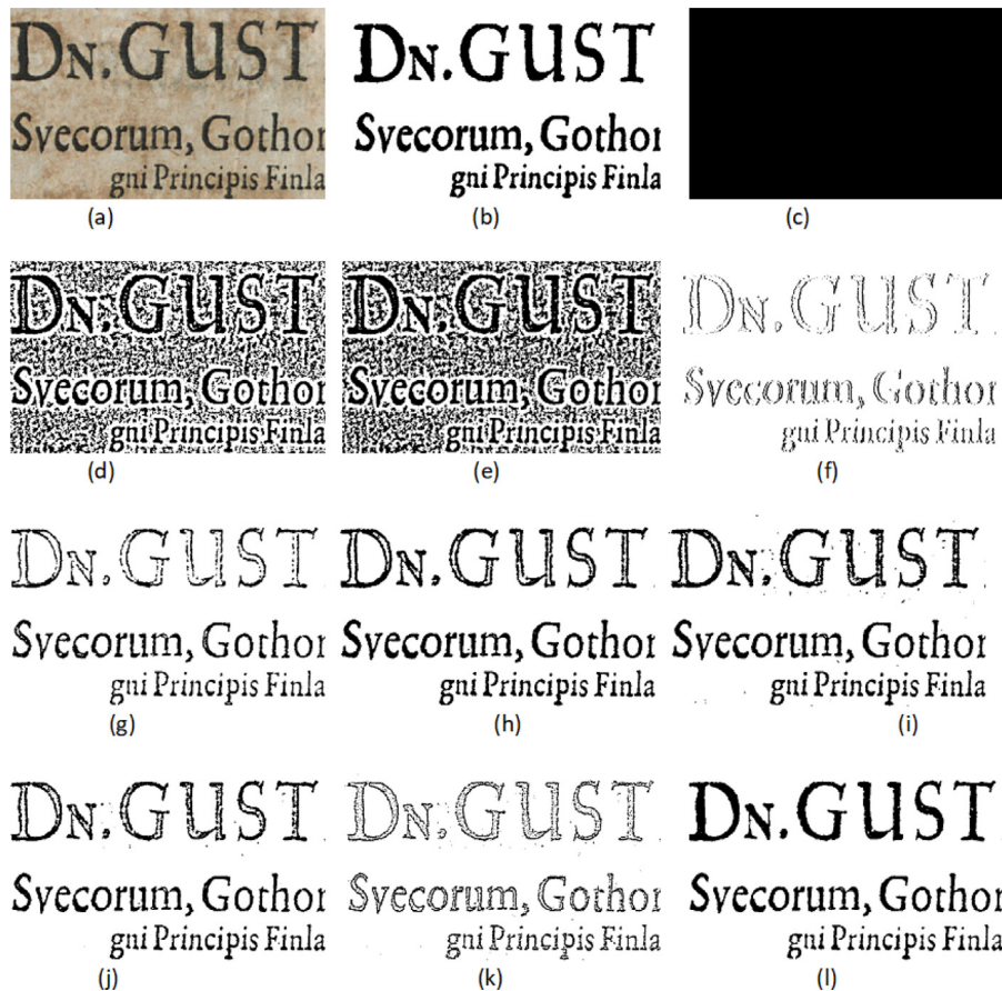
Fig. 5. (a) Part of image PR4.png from DIBCO-2011 dataset (Heavy and variable text stroke), (b) Ground truth, (c) Otsu, (d) Niblack, (e) Bernsen, (f) Wellner, (g) Sauvola, (h) Wolf, (i) Bradley & Roth, (j) NICK, (k) Singh et al. (2012), (l) Proposed.
