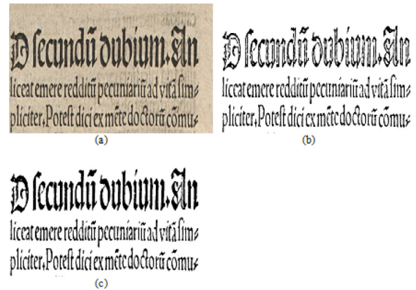
Fig. 3. (a) Input image (P02.bmp from DIBCO-2009), (b) Sauvola's output (F-measure = 77.14), (c) Proposed (F-measure = 91.72).
