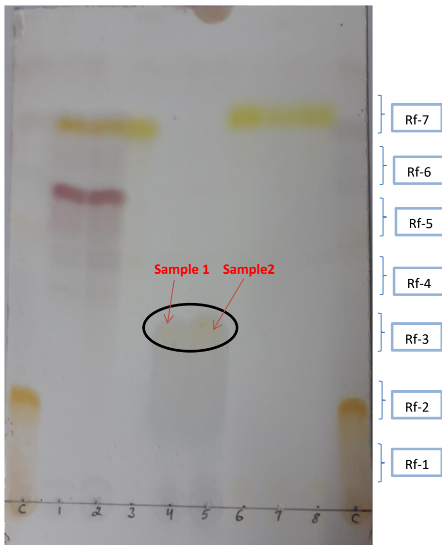
Figure 2. Showing TLC plate. The plate was ran using solvent system A for 40 minutes. Control sample (C) – Parmelinella wallichiana , spot 4 – Umbilicaria antarctica , and spot 5 – Umbilicaria aprina .
