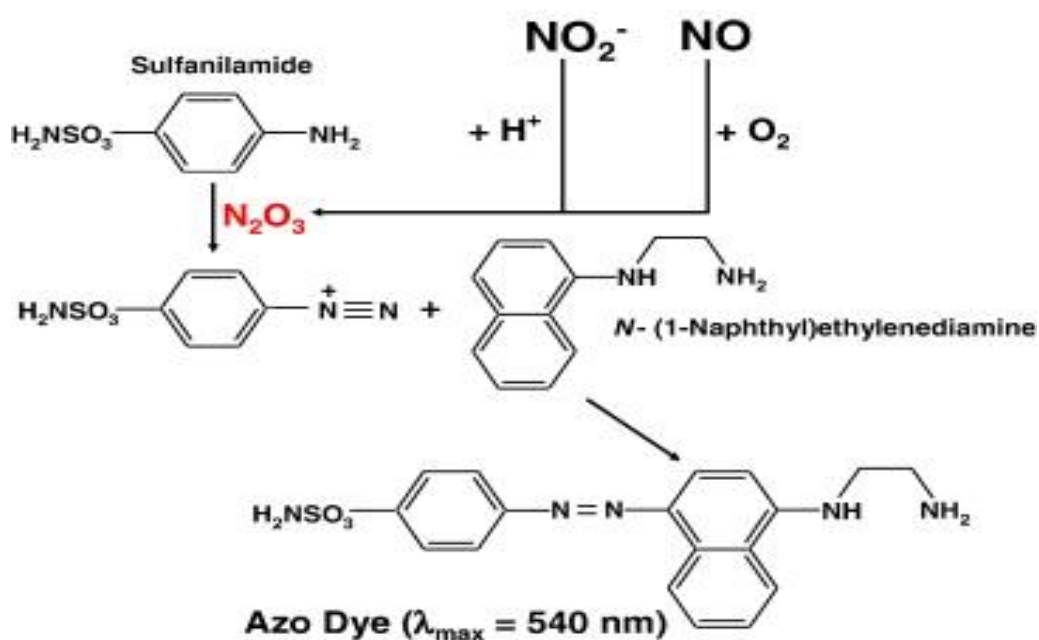
Figure 3.2: Reaction mechanism of NO detection (adapted from Elsevier.com)
