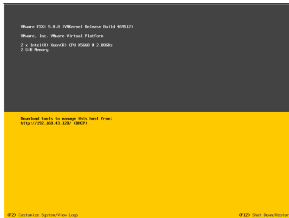
Figure C.12: VMWare ESXi Installed
