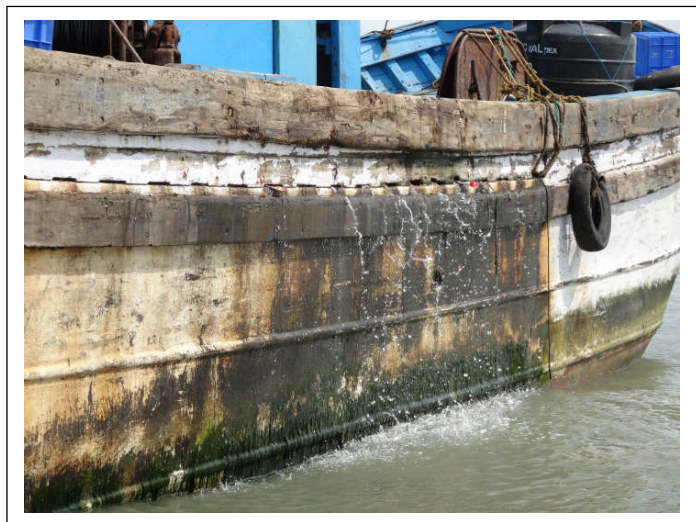
Figure 4. Fouling of the hull of a dinghy by Ulva paschima Bast, from Mangalore, Karnataka, May, 2012.
